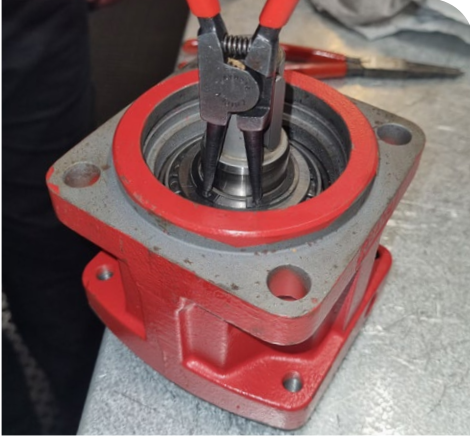
13. Disassemble the retaining ring (item 478)
