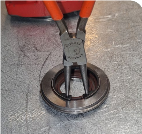
11. Disassemble the retaining ring (item 238)
