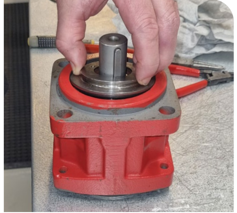
29. Install the seal carrier (item 231)
