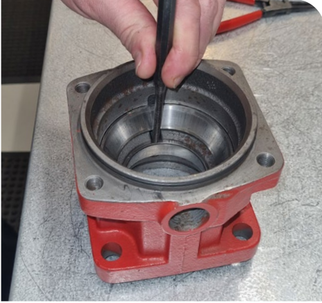
17. Tap the small bearing ring with a mandrel and hammer
