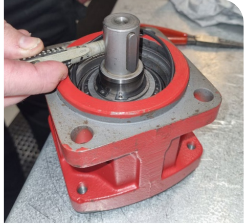
10. Remove the O-ring (item 225) Always change seal kit when removing seals.
