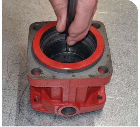
18. Tap the large bearing ring with a mandrel and hammer
