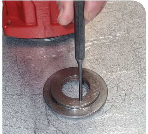
12. Tap the shaft seal out with hammer and mandrel.
