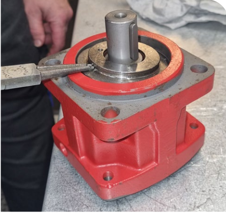
9. Remove the seal carrier (item 231)
