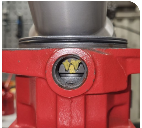
31. Install the O-ring (item 221) Included in seal kit
