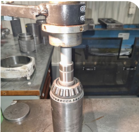
19. Place the ring gear (item 453) on a tube. Press out the shaft (item 311) by pressing on the shaft end.
