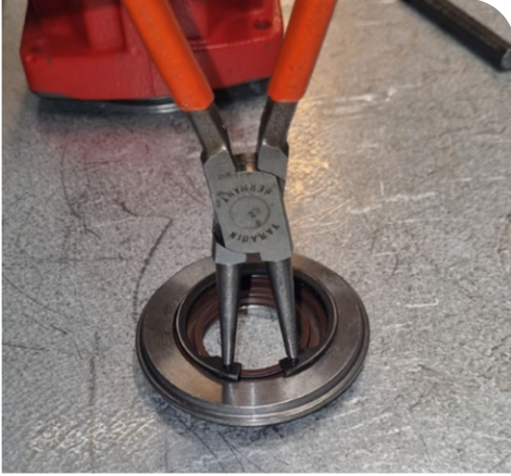
28. Assemble the retaining ring (item 238)
