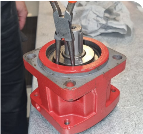
30. Install the retaining ring (item 237) Included in seal kit Tips! Tap with mandrel and hammer to secure retaining ring is correct assembled.
