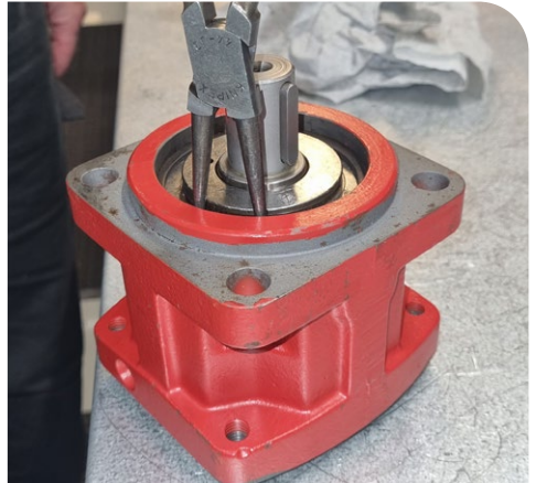
8. Disassemble the retaining ring (item 237)
